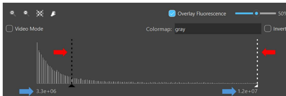
Figure 3-10 Two ways of setting the histogram limits. Set the lower or higher histogram limits by moving the black or white vertical bars (red arrows). Set the lower and higher limit values by double-clicking on the tick labels (blue arrows).
